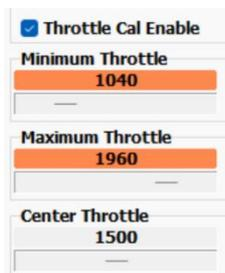
Before the first time you use GOV mode, reset the transmitter throttle range and perform throttle channel calibration (only once)
